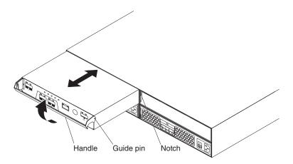
Figure 56. Reinstalling the controller
